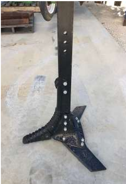
Figure 3: Ripper point with adjustable cultivating knives fitted.
