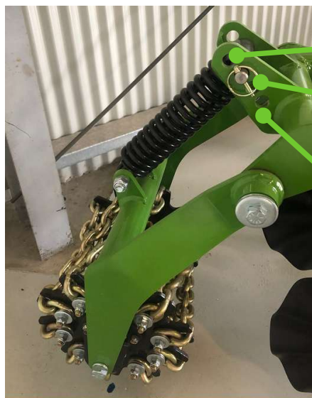
Figure 2: Optional Chain crumble roller shown here.
