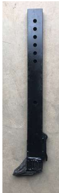
Figure 4: Minimum till tyne with spear point.
