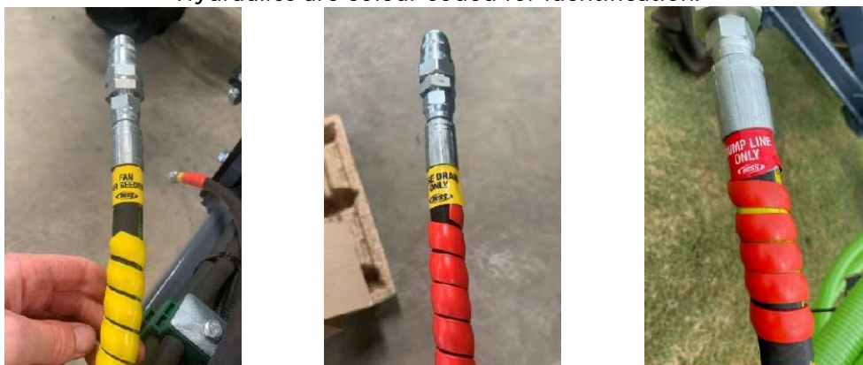
ISOBUS compatible Connection Plug and hydraulic lines. Hydraulics are colour coded for identification.
