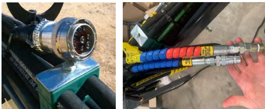
ISOBUS compatible Connection Plug and hydraulic lines. Hydraulics are colour coded for identification.
