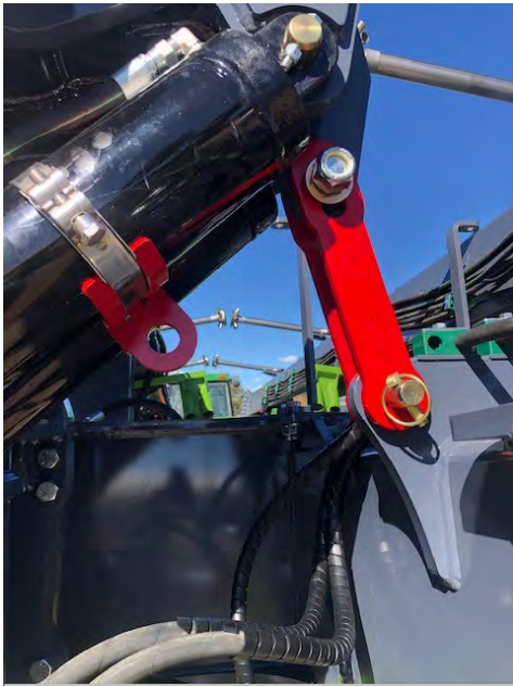
Locked for Transport
