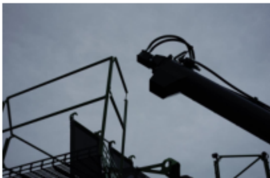
Be very mindful of overhead obstacles, particularly catwalks & Power Lines. Do not operate without safety screen on auger.
