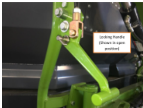
4.2.1 – Unlatch auger transport latches.
