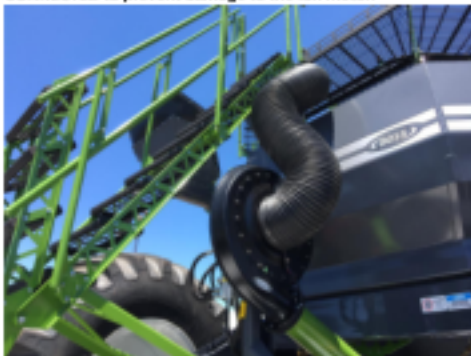
19s blower fan complete with remote intake and strainer
