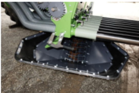
4.3.2 – Position hopper under bin to be emptied and flip rubber skirt up
