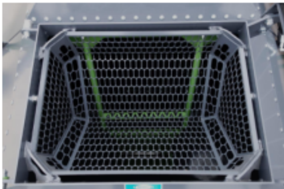
4.2.4 – Check bin fill strainers for cleanliness. Remove strainer to check inside bin and metering unit. Remove any foreign matter that could cause blockages.
