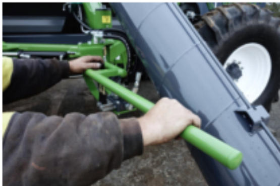
4.2.6 Operate controls with left hand, while steering extension bar with the right.
