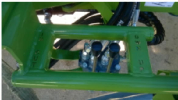
4.2.5 – Position auger using remote controls. The auger can be positioned for both bin filling and emptying
