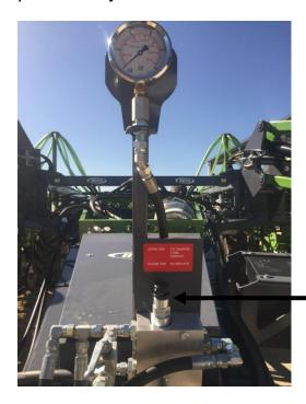
To adjust the systems operating pressure engage continuous oil flow, undo locking nut and screw in to increase or out to decrease operating pressure. When finished secure the locknut to maintain selected pressure setting.
