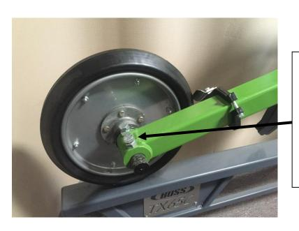
To adjust the press wheels in & out loosen the 2 locknuts & positioning bolts and slide the assembly to the required position ensuring the bolts and lock nuts are done up firmly once in position.
