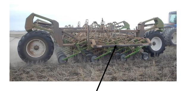
Ensure the frame or toolbar is running as level as possible and is parallel to the ground.
