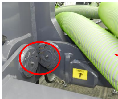
Frame & Drawbar Pivots – Grease Daily
