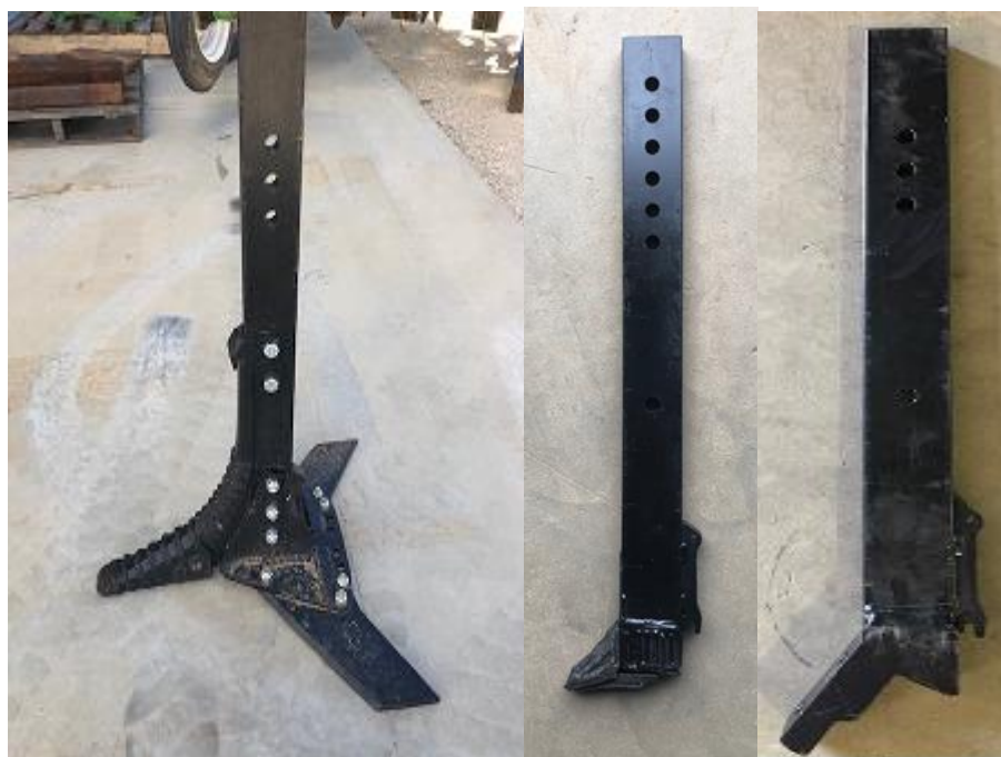
Ripper point with adjustable cultivating knives fitted.
