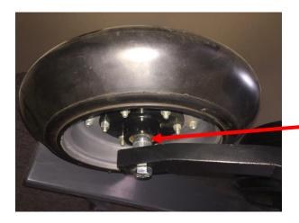
Remove the press wheel and add or remove shims as required. The press wheel is generally set away from the opening slot as this tends to close the seed trench from the bottom up. When positioned right over the top of the trench the press wheel can seal at the top but leave air pockets underneath (this depends on planting depth).
