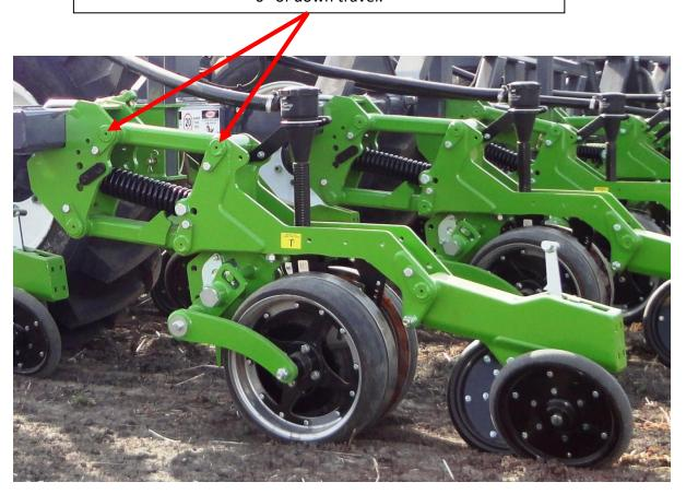
Ensure the main toolbar angle is set parallel to the ground. This can be checked visually by looking at the main RHS that the row unit mounts to, and making sure it is operating parallel to the ground when the unit is in the working position.
