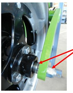
Undo the gauge wheel mounting bolt and add or remove shims as required so the gauge wheel lightly touches against the disc at the soil contact point.
