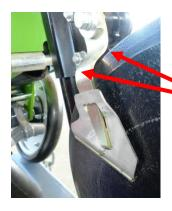
Ensure the scraper arm is low enough so when the machine is lifted and the gauge wheels drops down it cannot contact the arm, also check the scraper arm has clearance on the disc.
