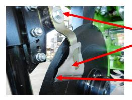
Loosen the mud scraper mounting bolt and remove the scraper blade.
