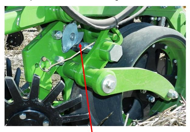
Check that the gauge wheel link arm is touching the depth cam to ensure set planting depth is being maintained.
