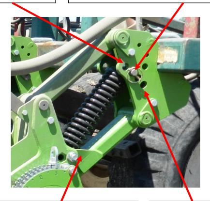
Lift the machine up so that the row unit sits on the down stop, before attempting to remove the adjustable pin.
