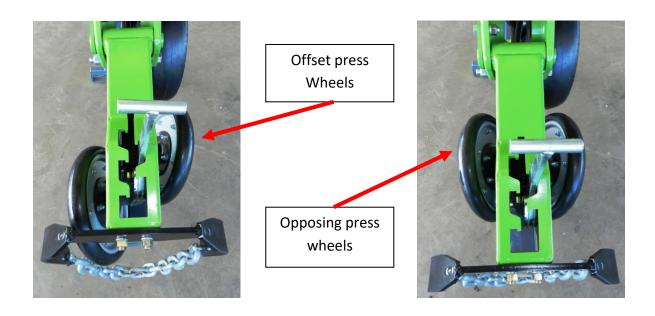
To change between offset and opposing press wheel settings remove both press wheels from the row unit. Remove the lockout bolt from the stowage position and relocate to the bottom hole position, ensuring it locates through the cut out in the rocker assembly so the press wheels pivot together. Bolt the press wheels back on the rocker assembly in the opposing mount positions.
