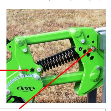
Lastly lift the row unit and replace the down-pressure spring into the lockout position. (Front pin is currently shown in the lockout position)
