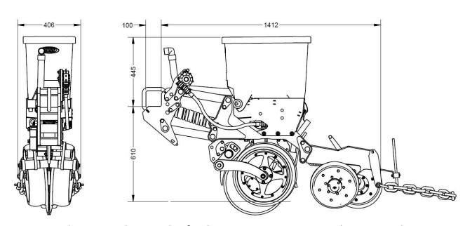
**DX50** working weight- 145kg for base row unit, Box, Whippers, Chains Extra.
