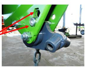
Make sure the lockout bolt has been placed through the cut out in the rocker assembly.
