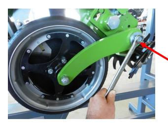
Remove the gauge wheel retaining bolt and slide the gauge wheel off the main pivot shaft.
