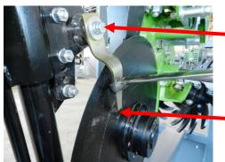
Retighten the scraper mounting bolt and place a ring spanner over the scraper arm and bend up or down until the tip of the arm lightly touches the disc. Now loosen the mounting bolt and put the scraper blade back on. Blade pressure can be varied this way as required when operating in different soil types.
