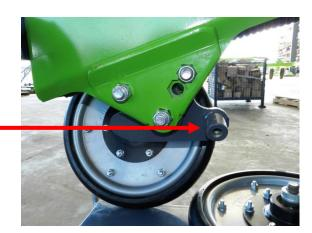
Remove the lockout bolt from stowage position & relocate to the bottom hole so the walking assembly becomes fixed. (Failure to do this will cause excessive wear to the press wheel tyre)
