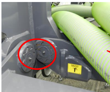
Frame & Drawbar Pivots – Grease Daily
